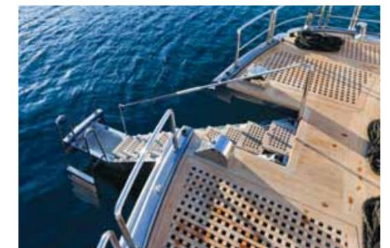
The Merlin design emphasises clean, open deck spaces, including an open air dining area in front of the main mast (above). At the stern on the main deck is an external hydraulic gangway, which drops to form a boarding and bathing platform (right)
